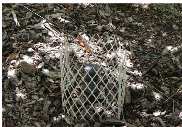
Protected soil moisture probe installed permanently in a grape orchard
