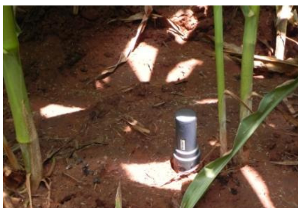
DACOM soil moisture probe in maize field
