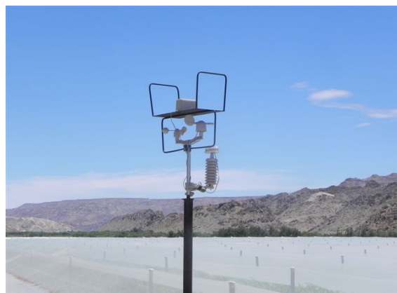
Weather station integrated with the "Irricheck" logging system for automated irrigation.
